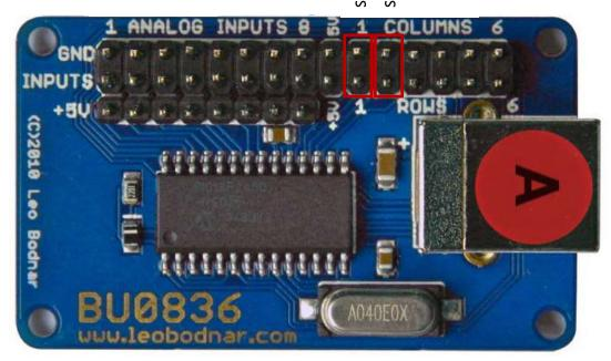
Once you have connected everything you need - connect to a PC or Mac using a standard USB A to B cable and the device will be recognised as a generic game device. You can then either calibrate or assign your controls using your chosen game or software as you would with any other game controller. That's it!
